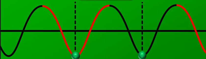
The diagram shows a continuous wave moving to the right. The wave is shown in black and red. Below the wave, particles are shown oscillating vertically. A yellow box contains the equation  $x = vt \rightarrow \lambda = vT \rightarrow \lambda = \frac{v}{f}$ .
